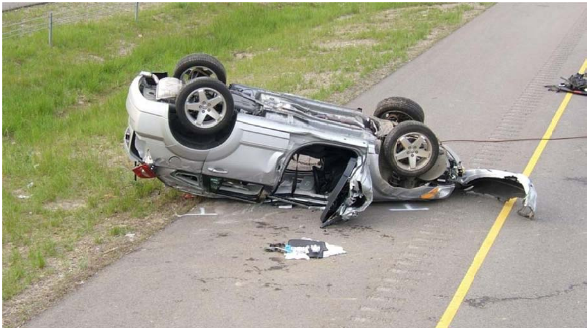
Figure 126. Example Rollover Crash Caused by High Redirection on Back Slope
