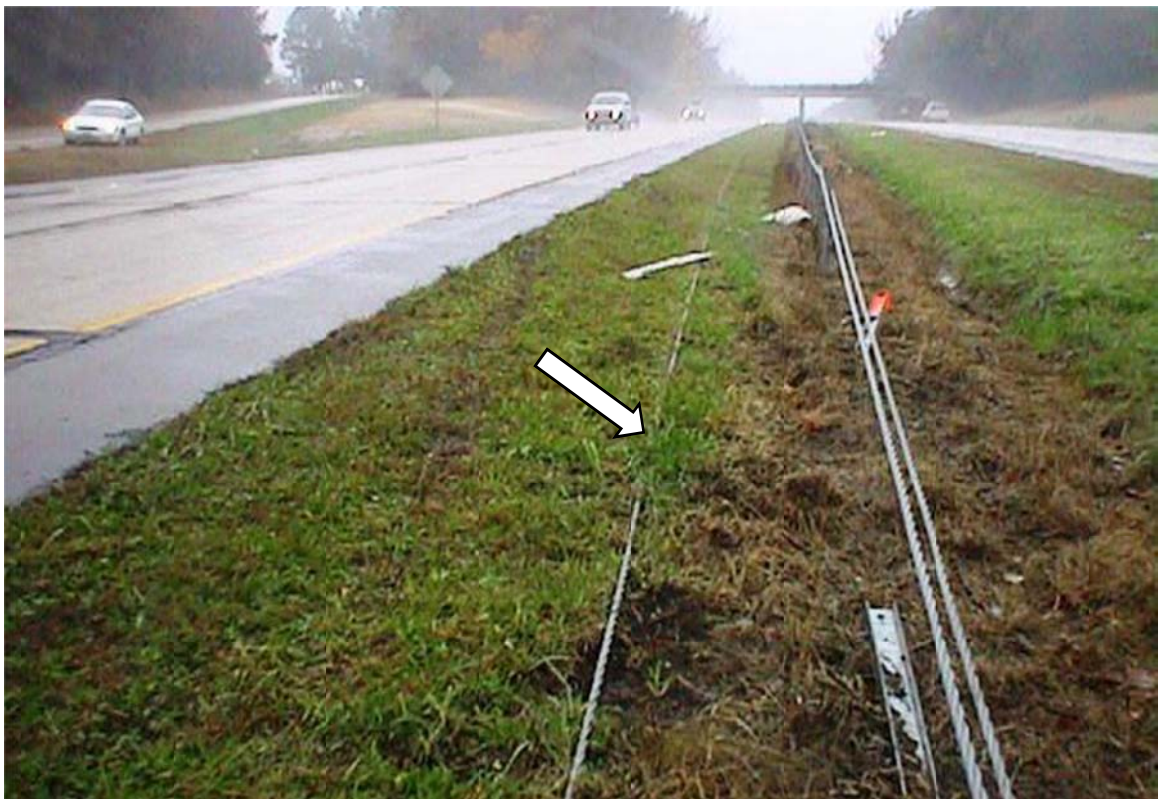
Figure 98. Back Side (Middle) Cable Release from Many Downstream Posts Resulting in Penetration
