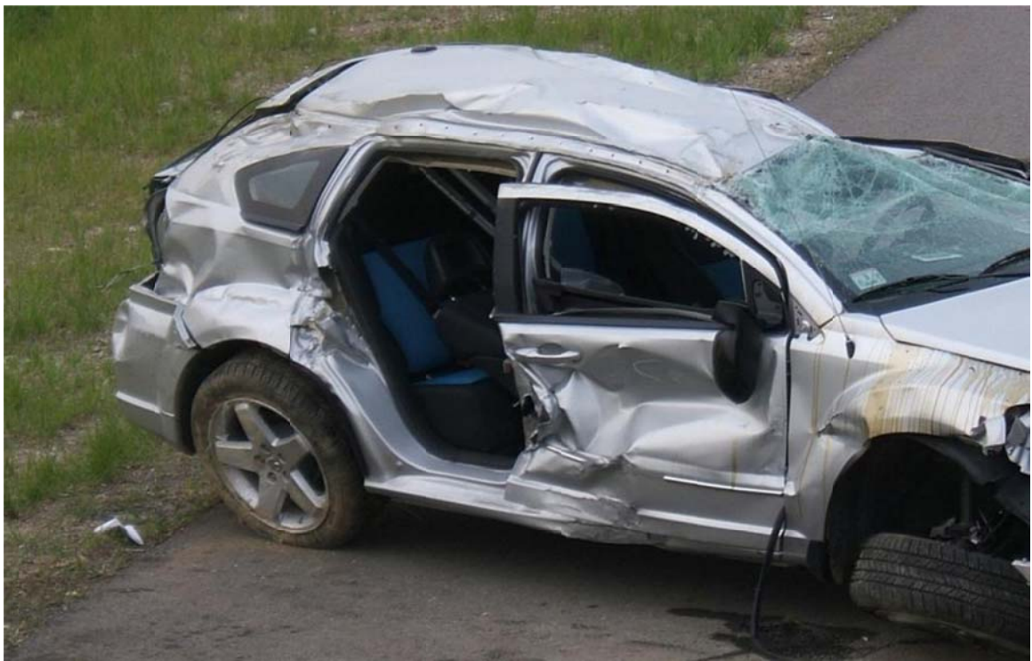
Figure 127. Example Rollover Crash Caused by Redirection on Back Slope (continued)
