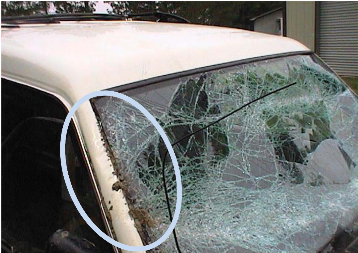
Figure 101. Brush Guard Prying Penetration with Cable Contact Striations on A-Pillar
