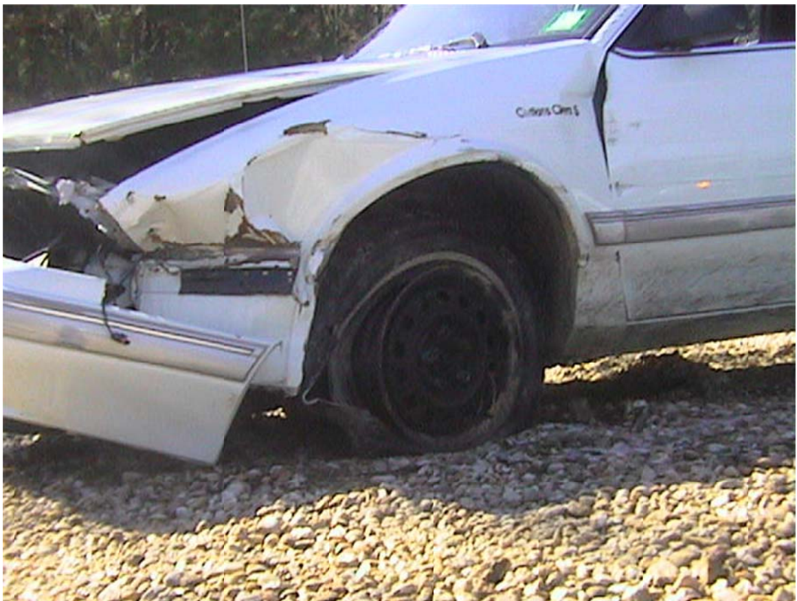
Figure 103. High-Tension Splice Tearout Penetration
