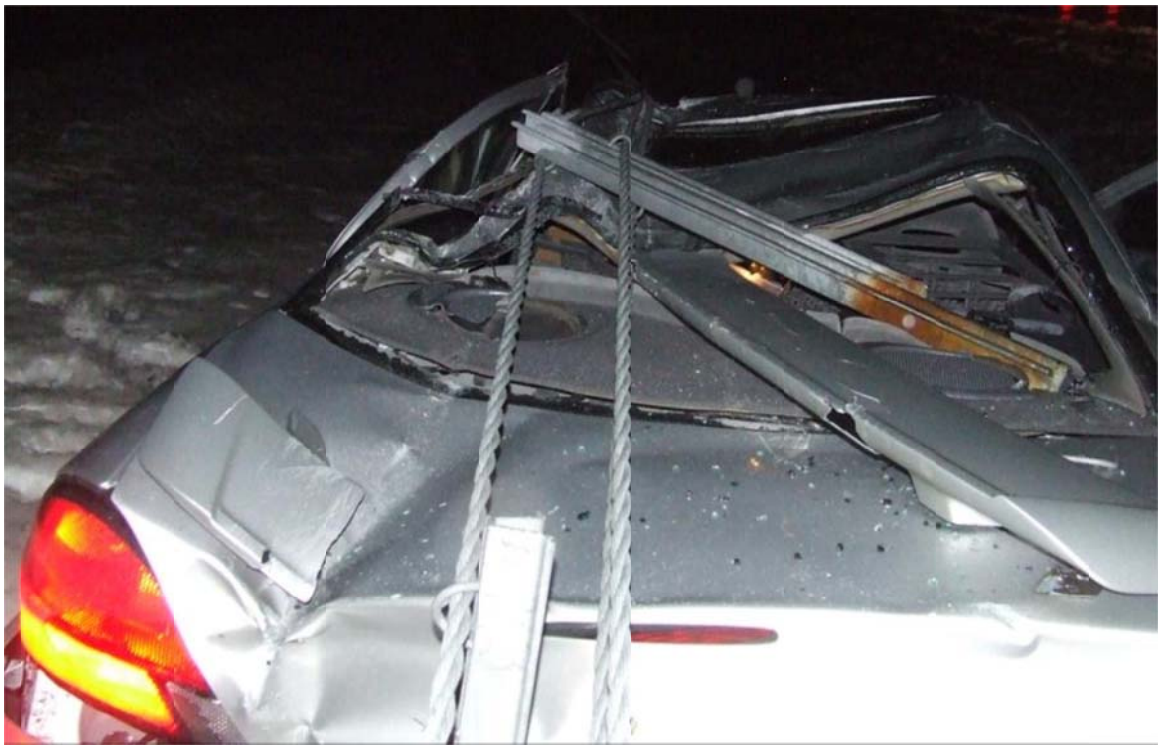
Figure 87. Potential Penetration Crash on Nucor NU-CABLE Barrier
